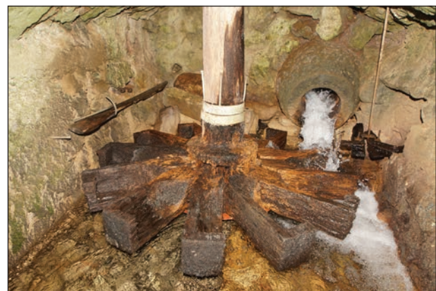
Figure 17: Wooden propeller used as a turbine for a mill in Konavle, Croatia, still in use. The same can be seen in Popovo Polje in Herzegovina, BiH (Photo: B. Juvanec).
